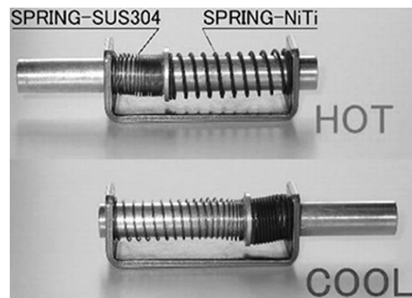
Fig. 3. Two way action actuator [6]. A SMA spring and a stainless steel spring are mounted in a holder working one against the other. When the SMA spring is heated it recovers its initial shape pushing the holder and deforming the stainless steel spring; during cooling the stainless steel spring retracts the holder deforming the SMA spring.
