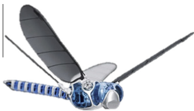
Fig. 18. Festo BionicOpter – inspiration dragonfly flight [286].
